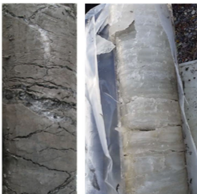
Permafrost cores with ice-rich silty clay (left) and massive ground ice (right)
